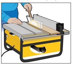
If width of last plank is less than 2.5", balance by cutting (Rip) last row of planks accordingly.
