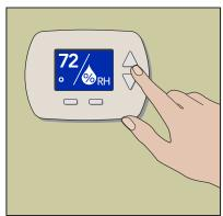
**Maintain** Environment Indoor relative humidity should be maintained with no more than a 30% fluctuation (E.g.30% -60%). Fluctuation of interior RH of more than 30% will likely result in gaps or bucking.
