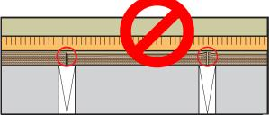
Improper substrate or flatness can result in gaps, squeaks, premature wear on surface and poor plank fitting during assembly.
