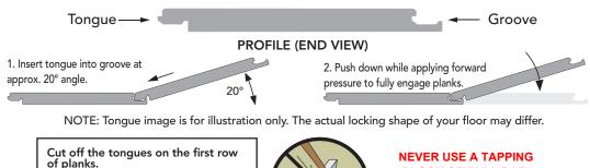
Be sure locking system is fully engaged! Planks must be flat in relation to each other (on all sides) without gaps before continuing installation.
