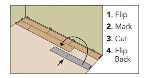
Power miter saw, table, circular and jig saws can be used to cut this flooring product.
