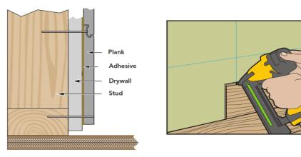
Use a level to double-check the levelness of the line between the two marks. Adjust line as needed with spacers. Secure this first row fully using adhesive and 2' finish nails or wood screws into pre-marked wall studs, placed approximately 2" above subfloor (these will be covered by your baseboard trim).
