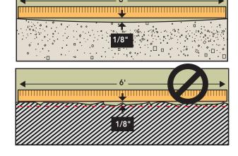
Improper substrate or flatness can result in gaps, locking mechanism failure and premature wear on surface.
