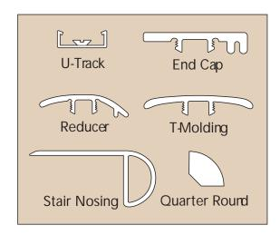
Quarter Round moldings are used to cover expansion spaces between the baseboards and the flooring.
