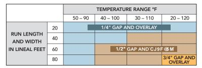
The temperature range is the actual temperature of the flooring which is affected by the substrate, sunlight and ambient temperature.
