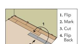
This material can be cut using a sharp utility knife & straight edge.
