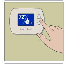
**Maintain** Environment After installation, maintain your flooring between the temperature ranges of 60°F - 80°F.
