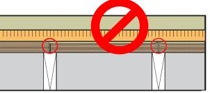
Improper substrate or flatness can result in gaps, squeaks, premature wear on surface and poor plank fitting during assembly.
