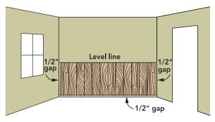
Trim out walls using 3/4" round (avoid nailing into planks). Install baseboard to cover gap along floor and Install threshold along top edge to finish wainscot wall.
