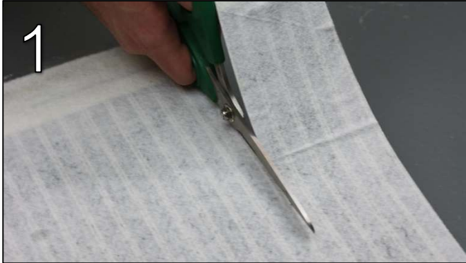
1 Cut between solid black bars all the way across the mat at the length needed.
