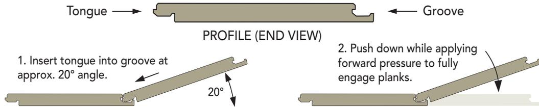
Cut off the tongues on the first row of planks. Be sure locking system is fully engaged! Planks must be flat in relation to each other (on all sides) without gaps before continuing installation.
