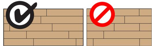
**STEP 10. Continue installing each additional row as shown until area is completed.**
