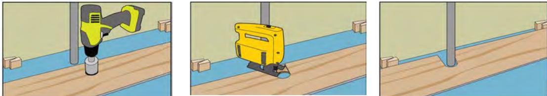
When there is single pipe on a wall, you can plan to have the end-joints meet at pipe, drill and install as shown.
