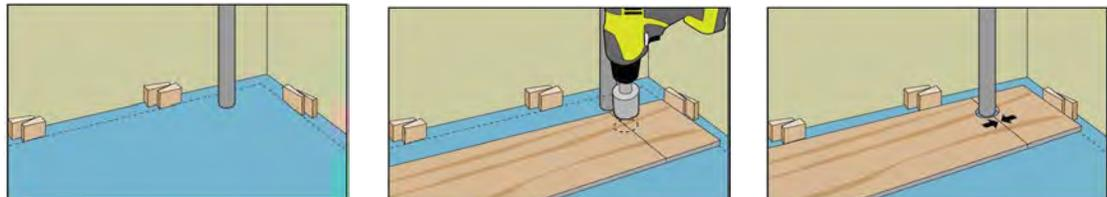
If there are multiple or larger pipes passing through the floor make hole(s) on the plank 3/4" greater than the diameter of the pipe, cut the plank with a 45° angle towards the hole. The cut-off piece edges are glued in the position again. *Do not glue to the subfloor.*
