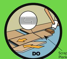
Use Scrap Plank To Align, Then Tapping Block On Short Edge Until Secure. (Never Hammer Directly On Plank)
