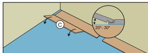
Install remaining planks of the first row by first inserting their long edge tongue to the guide plank's long edge groove, but before lowering it ensure it is approx. 3/16" away from the previous installed plank. To connect the planks, use plank section A. combined with a tap block\* and hammer lightly tap (use Plank Section A) the new plank's short end groove until it is fully connected with the previous plank.
