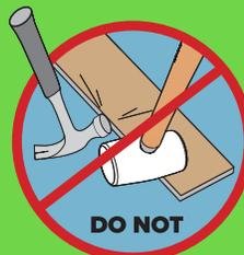
Never Tap, Hammer Or Use Mallets On Long Edge of Planks
