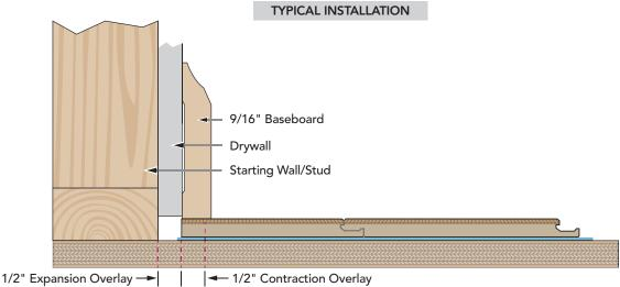
How to achieve required Expansion Gap / Contraction Overlay using base board only
