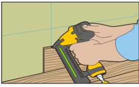
Use a level to double-check the levelness of the line between the two marks. Adjust line as needed with spacers. Secure this first row fully using adhesive and 2' finish nails or wood screws into pre-marked wall studs, placed approximately 2" above subfloor (these will be covered by your baseboard trim).
