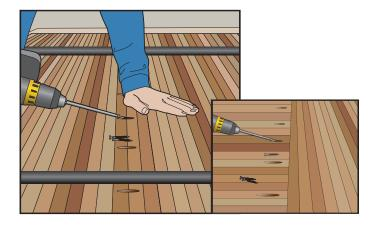
*Miter bolts* are typically used to hold the corner pieces together but also for sides and end joint connections. Lay the pieces topside down, and line up the reference mark for the corner. Draw marks across each seam for the miter bolts.
