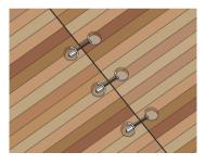
Biscuit Joinery: A biscuit joiner (also known as a plate joiner) cuts half-oval slots in mating workpieces; then you glue in a football-shaped "biscuit" and clamp the joint tightly. Biscuits add strength to joints and assist you in aligning workpieces.
