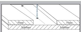
Draw a line down the center of the space between floors. Drill 1/4" holes along the line, approximately 15" apart, starting 2" from each side.
