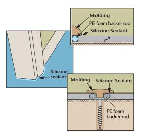
To ensure the floor is able to "float" freely, be sure to affix baseboards or moldings to the walls, not to the floors. This way, the floor can expand & contract within the gap.
