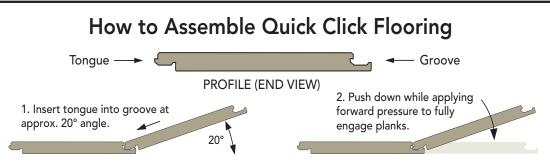
Cut off the tongues on the first row of planks. Be sure locking system is fully engaged! Planks must be flat in relation to each other (on all sides) without gaps before continuing installation.
