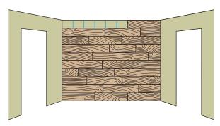
• The last row will need to be cut lengthwise (ripped down) to fit properly to the ceiling, leaving a minimum 1/2" for expansion.
