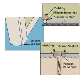
To ensure the floor is able to "float" freely, be sure to affix baseboards or moldings to the walls, not to the floors. This way, the floor can expand & contract within the gap.
