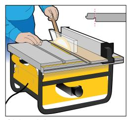
If width of last plank is less than 2.5", balance by cutting (Rip) starting row of planks accordingly.
