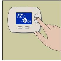
**Maintain** Environment Indoor relative humidity should be maintained with no more than a 30% fluctuation (E.g. 30% -60%). Indoor Relative Humidity levels below 30% or above 70% will likely result in gaps or bucking.
