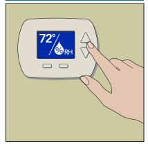
**Maintain** Environment Indoor relative humidity should be maintained with no more than a 30% fluctuation (E.g. 30% -60%). Indoor Relative Humidity levels below 30% or above 70% will likely result in gaps or bucking.
