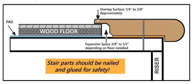
If there is an existing "overhanging" stair nosing, you must cut it off before installing the overlap stair nosing. Trim off to the riser line as shown below:
