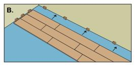
Spacers:Use spacers to maintain a minimum 1/2" expansion gap between the flooring and the walls. Place spacers adjacent to each plank joint and at the beginning and end of each row. This will lock-in assembled panels and prevent shifting during installation.
