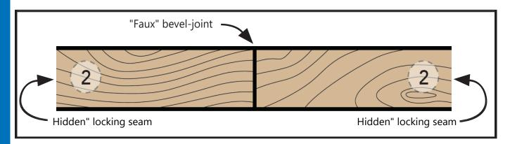
In each box you will find 3 types of planks (5 pcs./box), each is numbered on the back as shown: IMPORTANT NOTE: 1 will always join 1 and 2 will always join 2!
