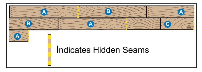
How to start rows using full plank then 1/3rd and 2/3rd cut planks.
