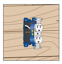
Do not cover receptacle retaining screw /surrounding fixture, to allow for bringing receptacle forward to accommodate for the thickness of new planks.
