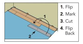
The piece you cut off may be used as the first piece in the next row, if it meets the minimum length criteria for the pattern being installed.
