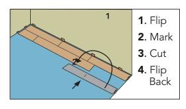
The best method for cutting this flooring is to use a power miter saw.
