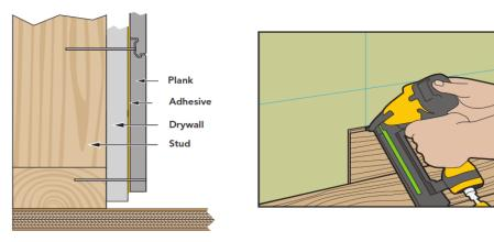
Use a level to double-check the levelness of the line between the two marks. Adjust line as needed with spacers. Secure this first row fully using adhesive and 2' finish nails or wood screws into pre-marked wall studs, placed approximately 2" above subfloor (these will be covered by your baseboard trim).
