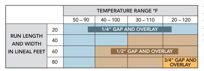
The temperature range is the actual temperature of the flooring which is affected by the substrate, sunlight and ambient temperature.
