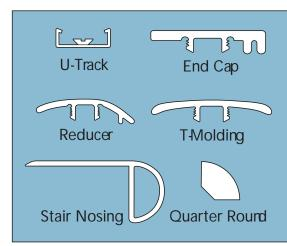
Quarter Round moldings are used to cover expansion spaces between the baseboards and the flooring.
