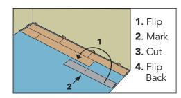
The best method for cutting Coreluxe flooring is to use a power miter saw.
