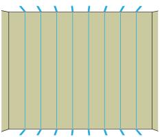
• Using a chalk line stretched between bottom and top mark, snap a line. Use painters tape at top & bottom of **each** stud on floor and ceiling to identify nailing points.
