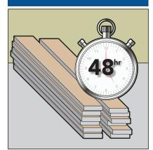
**Acclimate** Completely Acclimate your flooring to interior temperature for at least 48 hours. Temp. must be between 50°F – 85°F.
