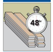
**Acclimate** Completely Acclimate your flooring to interior temperature for at least 48 hours. Temp. must be between 50°F – 85°F.
