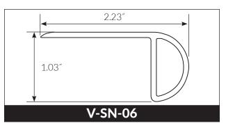
Surface Laminate: Wear resistant laminate | Core Material: Rigid PVC
